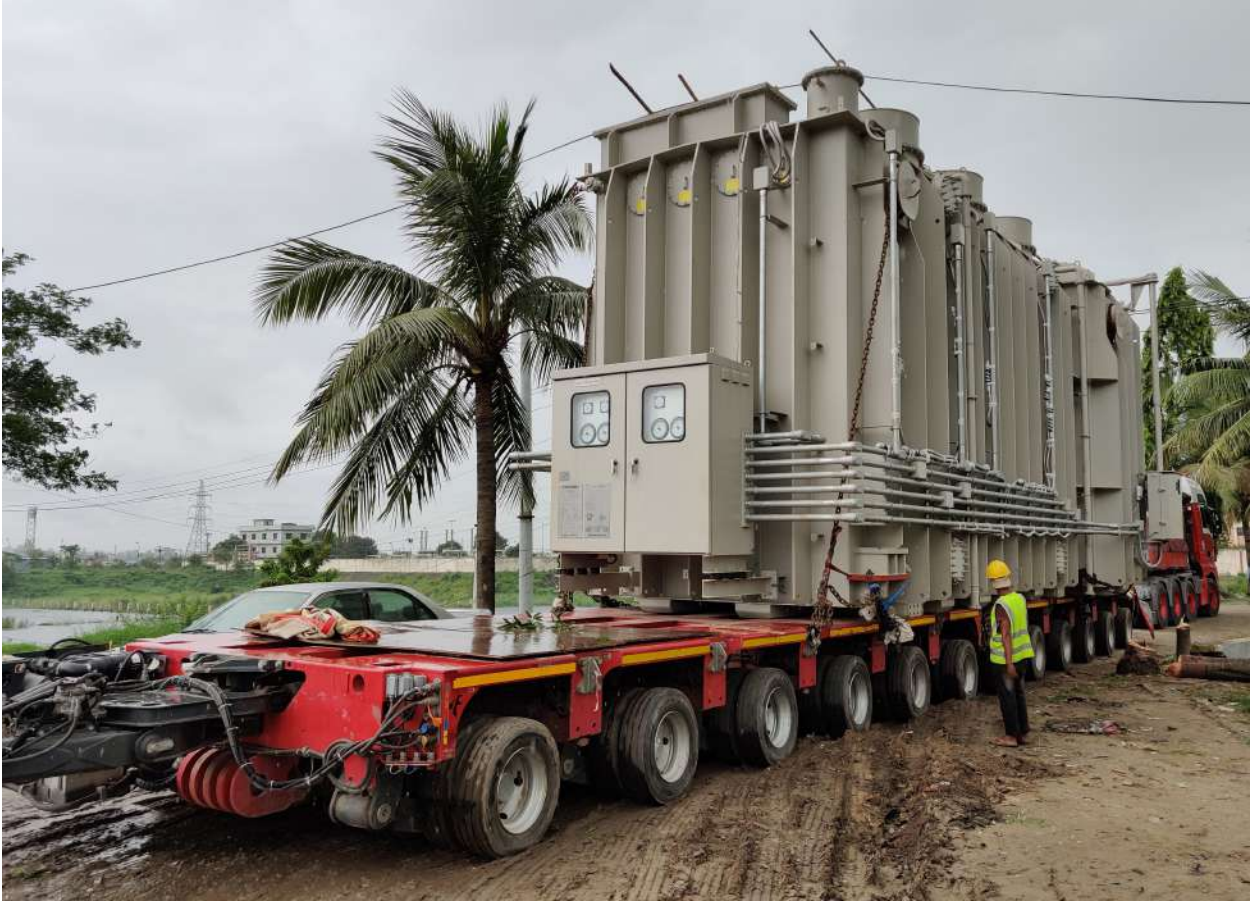
Picture 06 : Inland transportation using modular trailer.
