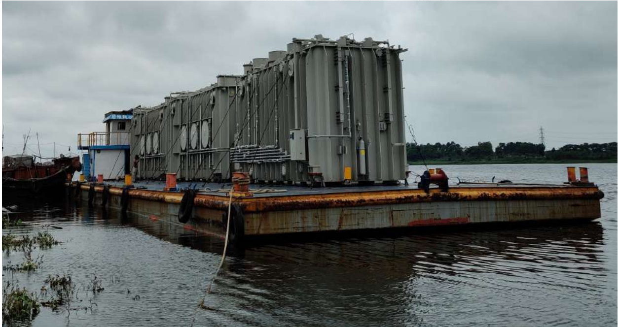
Picture 03 : Waterway transportation using barge.
