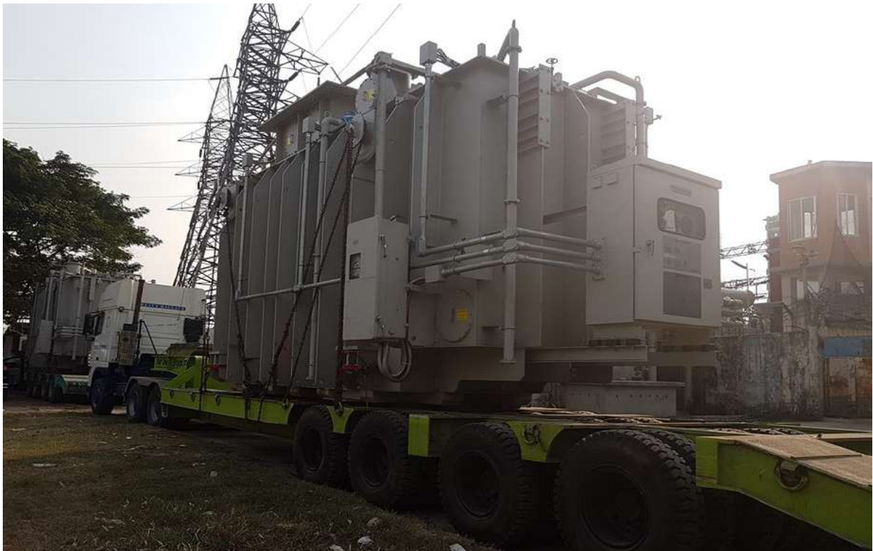
Picture 08 : Inland transportation using low-bed trailer.
