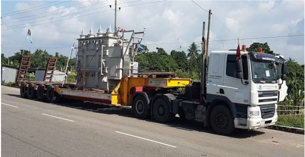
Picture 07 : Inland transportation using low-bed trailer.
